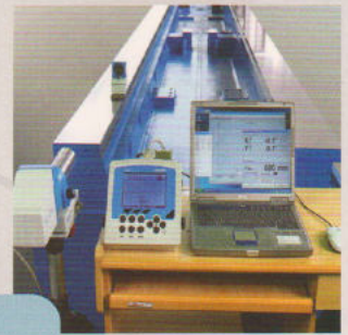
Straightness inspection with collimator
