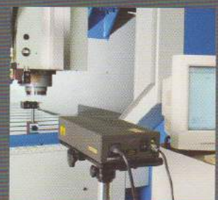
▲ Positioning accuracy inspection ISO 10791-4
