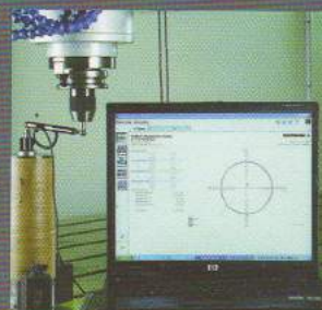
▲ 2-axis accuracy inspection ISO 10791-6
