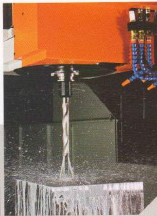
Mold cutting: Tool dia.:25mm Feed rate:5000mm/min
